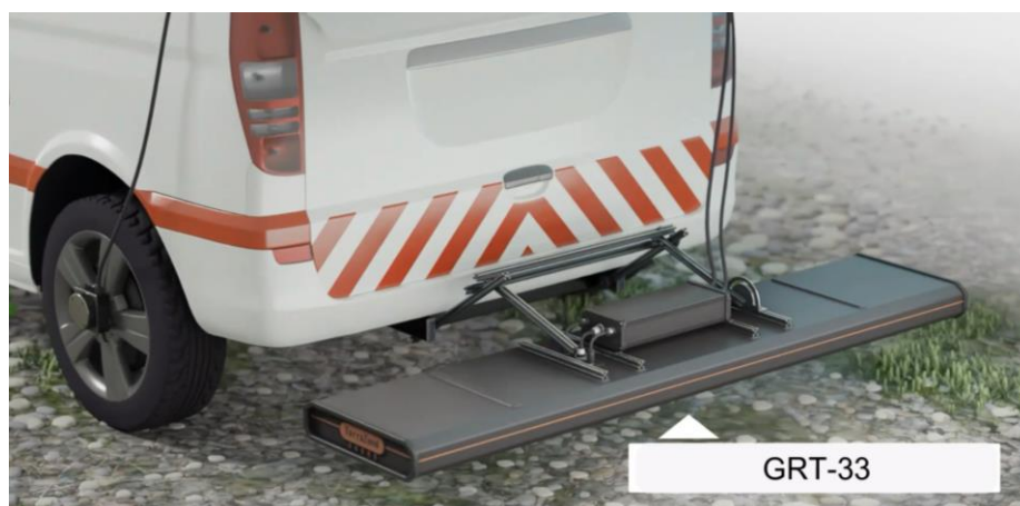
Figure 6. GPR mounting on a road car of a laboratory.
